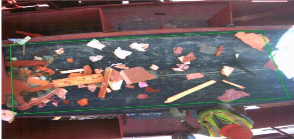
Real-time material detection and counting. Green boxes indicate detected and counted materials within the defined ROI
